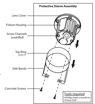
**4**- Please, support the fixture in the desired position using standard masonry proceedures.
